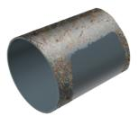
After determining where the sensors are to be installed, clean the pipe surface by removing dirt, rust and any roughness (paintwork is not a problem if it is in good condition).
