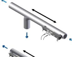
Reflex mode V: Distance > (3x) pipe diameter Direct mode / : Distance > (5x) pipe diameter
