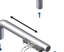
Reflex mode V : Distance > (15x) pipe diameter Direct mode / : Distance > (20x) pipe diameter
