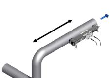
Reflex mode V: Distance > (3x) pipe diameter Direct mode / : Distance > (5x) pipe diameter
