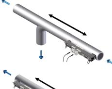
Reflex mode V : Distance > (3x) pipe diameter Direct mode / : Distance > (5x) pipe diameter
