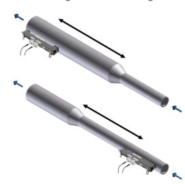
Reflex mode V : Distance > (30x) pipe diameter Direct mode / : Distance > (40x) pipe diameter
