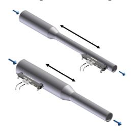
Reflex mode V : Distance > (10x) pipe diameter Direct mode / : Distance > (15x) pipe diameter
