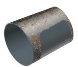
After determining where the sensors are to be installed, clean the pipe surface by removing dirt, rust and any roughness (paintwork is not a problem if it is in good condition).
