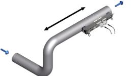
Reflex mode V : Distance > (15x) pipe diameter Direct mode / : Distance > (20x) pipe diameter
