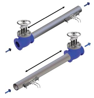
Reflex mode V : Distance > (15x) pipe diameter Direct mode / : Distance > (20x) pipe diameter
