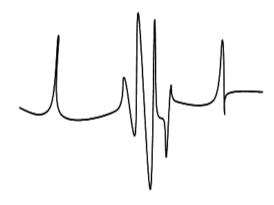
**Comment:** in this case, move the cables (in particular the probe cables) away from the power cables. Check the ground connections and the shielding.
