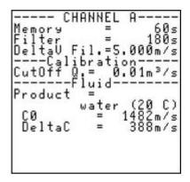
This feature must be used when the flow is extremely chaotic and an average for the flow needs to be produced in order to view its evolution.
