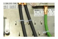
Use the loops pressed out of the metalwork to fit ties to secure the cables. There are two rows of loops available, to be used according to the number of ultrasonic chords connected, and also to secure other cables.
