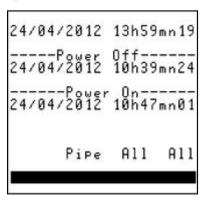
This screen indicates the date and time of the flow meter and the information concerning the last powering on.
