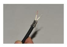
Unsheath a length of cable of between 10 and 15mm and bend back the ground braiding as shown opposite. Next, strip a length of about 5 mm of the conductors. Whilst doing this, note the colour difference of the two conductors: on the Twinax cable, the one is a galvanised colour and the other copper-coloured.
