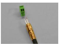
Cover the ground braiding with copper tape to prevent the threads of the ground from becoming loose and thus causing short-circuits. After passing it through the cable gland of your choice, connect the probe cable to the terminal board (disconnect the machine if this makes the operation easier), taking care always to connect the copper-coloured conductor on the same side on the terminals.
