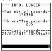
This page indicates the status of the logger and the last recording made.
