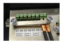
Only tighten the knurled nuts at the end, ensuring the shield connection jumpers are correctly secured, avoiding pressure exertion on the contact plates placed below these jumpers.
