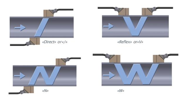
The preferred mounting method is the V-shaped mounting, which is suitable in most cases.
