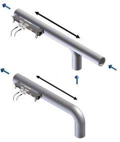
Reflex mode V : Distance > (15x) pipe diameter Direct mode / : Distance > (20x) pipe diameter
