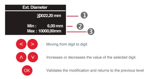
This type of screen allows entry all the numerical parameters in the device.
