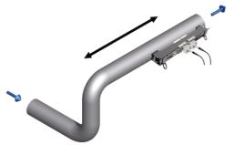
Reflex mode V : Distance > (15x) pipe diameter Direct mode / : Distance > (20x) pipe diameter
