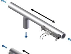
Reflex mode V : Distance > (3x) pipe diameter Direct mode / : Distance > (5x) pipe diameter
